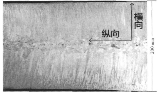
图 1 N08810 合金连铸板坯低倍组织及取样方向 Fig. 1 Macrostructure and sampling direction of casting slab of N08810 alloy
